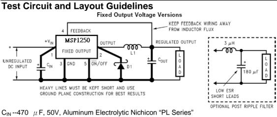
C<sub>IN</sub>--470  $\mu$  F, 50V, Aluminum Electrolytic Nichicon "PL Series" C<sub>OUT</sub> --220  $\mu$  F, 25V Aluminum Electrolytic, Nichicon "PL Series" D<sub>1</sub>--5A, 40V Schottky Rectifier, 1N5825 L<sub>1</sub> --68  $\mu$  H, L38
