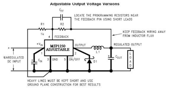
$$V_{OUT} = V_{REF} \left( 1 + \frac{R_2}{R_1} \right)$$
